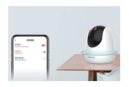
You can set the pan/tilt partol locations through the TDSEE App, and the camera rotates cyclically according to the preset location to patrol the area.
