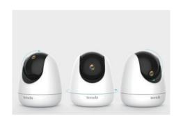
High speed pan/tilt design enables flexible rotation in all directions. CP6 covers 360° horizontally and 155° vertically (90° up, 65° down) which leave zero blind zones at all.
