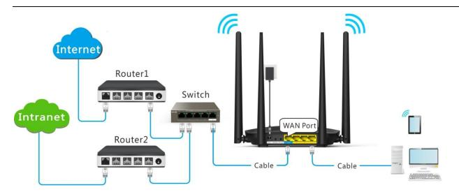
Router 1 accesses the internet and Router 2 the intranet. AC5 gets IP address to access the internet from Router 1 automatically. Set static route on AC5, achieving LAN clients access both internet and intranet.
